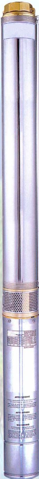
Electrical submersibles are with radial or semi-axial impellers. The impellers and the diffusers are in plastic material (noryl), whereas the bearings are in ceramic/rubber lubricated by the water circulation. Check valve is incorporated in the delivery body with threaded outlet. The coupling pump-motor is according to NEMA regulations.
